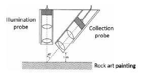
Figure 3. Measurement geometry used for microfade testing. The illumination probe is used to irradiate the material at a 0 degree angle, while the reflected light is collected by the observation probe using a 45 degree orientation relative to the sample (Diagram adapted from Whitmore et al., 1999)
