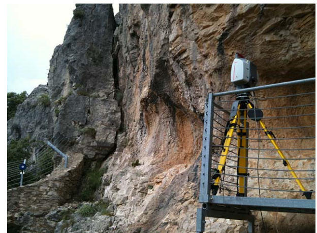
Figure 2. Terrestrial laser scanning setup targeting Shelters I and II
